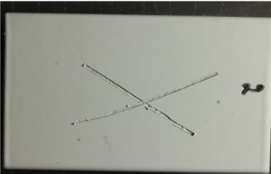
Fig. 10 - Sample 2 - Condition after 2000h AASS test
