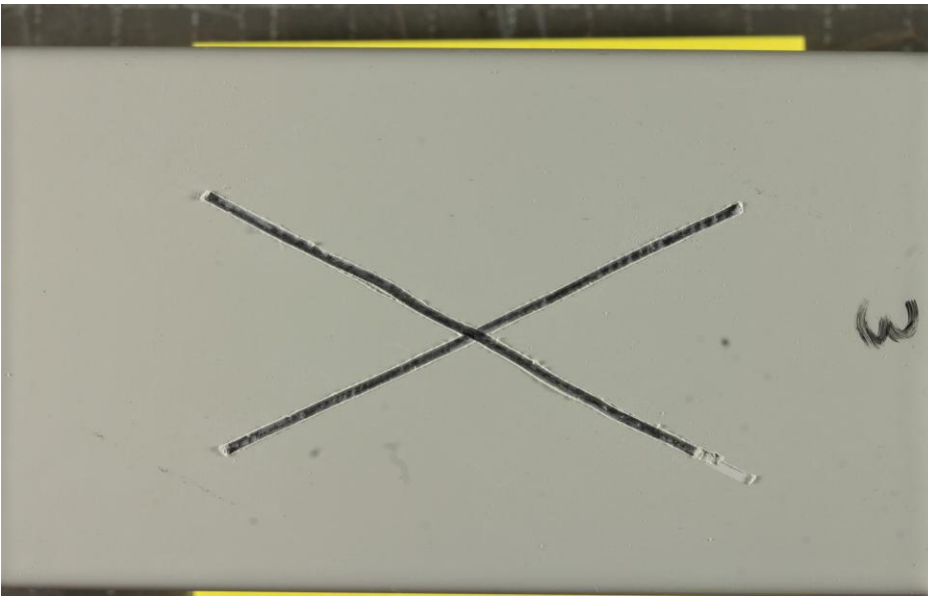
Fig. 3 - Sample 3 - Initial condition of the received samples (incl. scratch)
